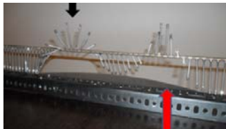
Fig. 1. Kink (black arrow) and antikink (red arrow) solitons rotate the pendulums from 0 to 2\pi (kink) or from 0 to -2\pi (antikink).
