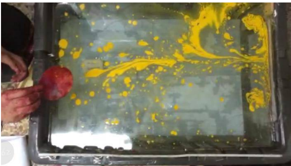
Fig. 1. Experiment shows if the vortices reach the wall they are scattered from each other
