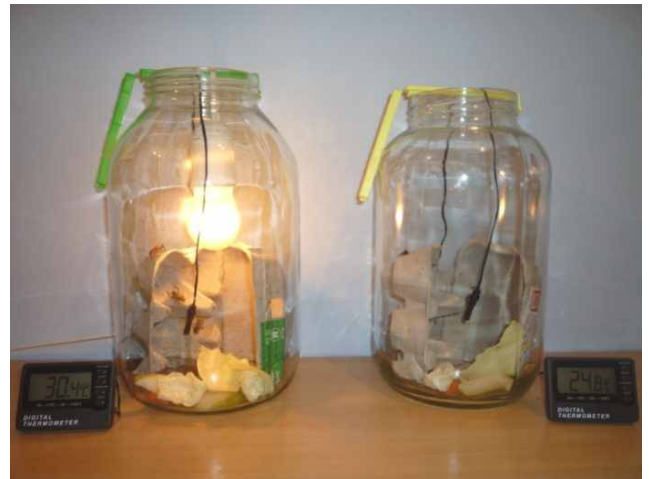
Figure 2. Study terrariums. The 15 W light bulb heated terrarium (left) assured an average temperature of 31°C, while at the unheated terrarium (right) an average temperature was 24°C.
