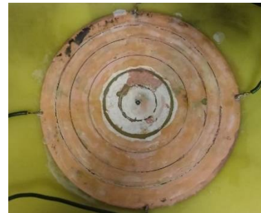
Fig. 3. The circular plate used for experiments. For examining the influence of holes on the results obtained using this method, a circular plate was
