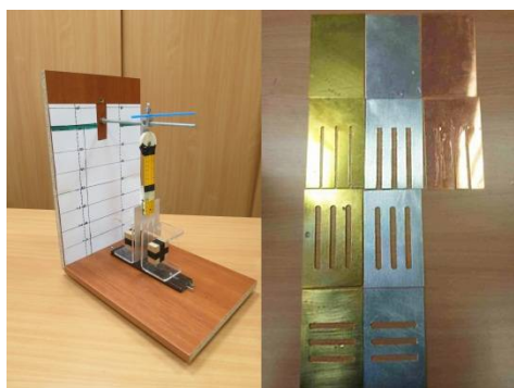
Figure 1 The pendulum and some of the plates (conductors) used in the experiment
