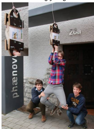
Fig. 1. Even my colleagues and I were not able to pull the interleaved phonebooks apart
