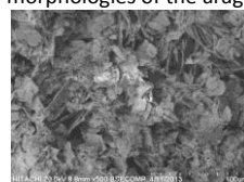
3.3: Scanning Electron Microscope Image CaCO 3 At 90 RPM
